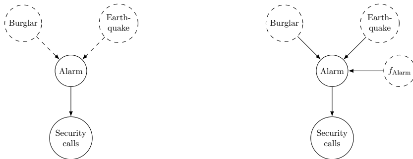
(a) Dashed-arrow representation of unknown causal relationships. (b) Unknown causal relationships represented in a latent function node f_{\text{Alarm}} .
