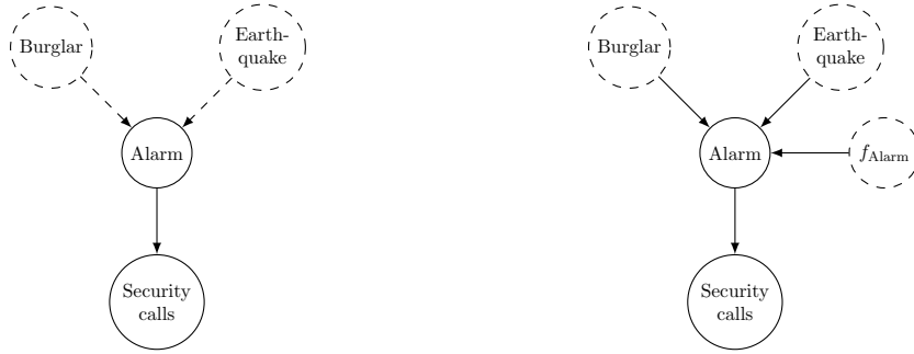
(a) Unknown causal relationships. (b) Unknown causal relationships represented in a latent function node f_{\text{Alarm}} .
