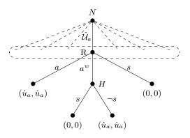
Figure 11.1.: The off-switch game modeled with a Harsanyi transformation. The dotted lines show the information set of R. Nature moves first by deciding the rules of the game, that is the utility  $\dot{u}_a$  of action a. H observes the move by Nature, but R does not.
