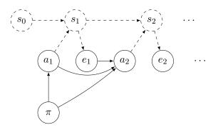
Figure 5.1.: Causal graph of the POMDP base. Here s, a, e, and  $\pi$  are as explained in Sections 5.1 and 5.2.
