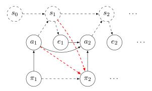
Figure 5.3.: Causal graph of a POMDP setup with an embedded agent. The agent's policy may be modified by the agent's own action and the state. It is often natural to think that the action causes the corruption with the state providing context.
