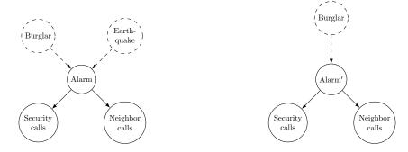
(a) Non-aggregated representation. (b) Earthquake aggregated with Alarm.
